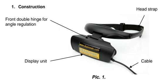
The goggles are powered from DVI socket which is located on the side of the scanner.
