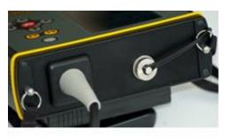
Photo 1a. Probe cable socket. PC transmission port
