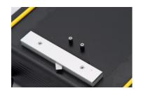
Photo 3. Strap and terminals for battery
