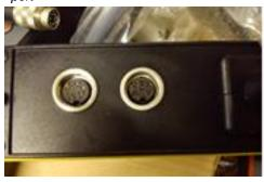
Photo 1b. Version with goggles. 5-pin socket for data transfer to a PC and 12-pin socket for goggles
